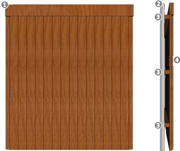
1: Top Rail; 2: Galvanized or Stainless-Steel Post (Recommended Minimum of 2.375"); 3: Stinger Board (Recommended Minimum of 2" x 3"); 4: Minimum 1/2" Wood Screen.
